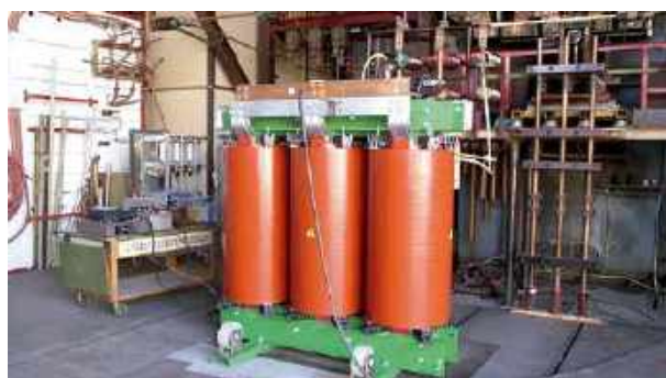
Short circuit test at CESI (MI)
