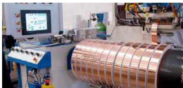
HV copper winding
